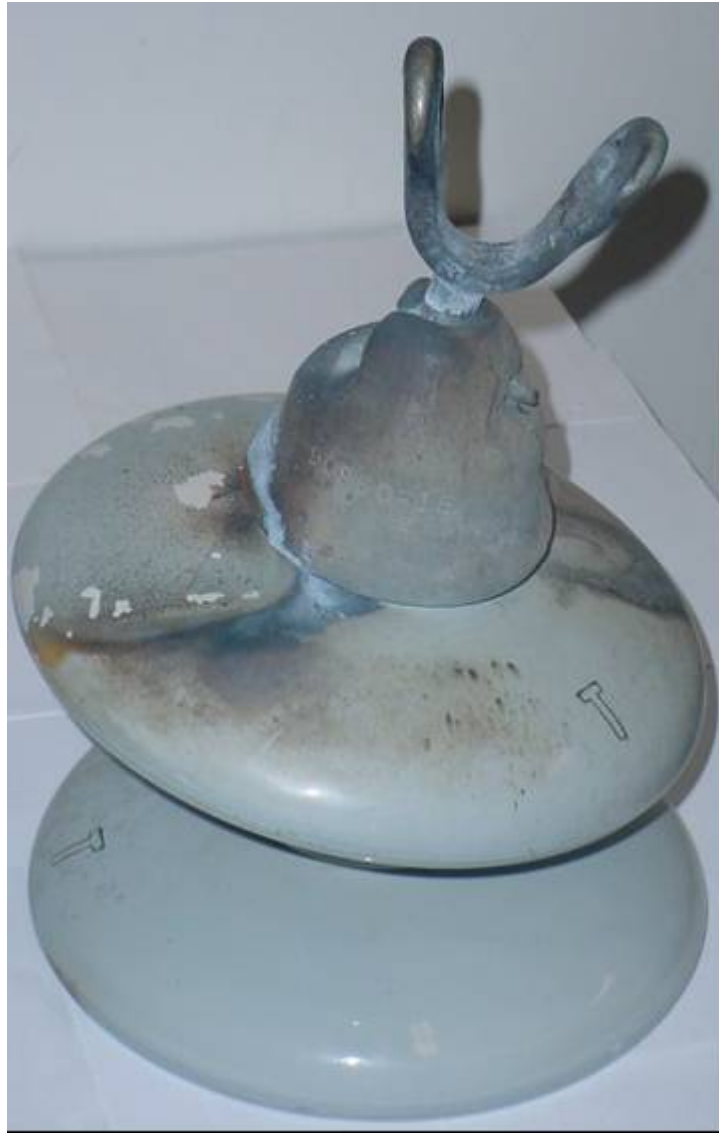
Fig. 4: Flashed porcelain cap and pin suspension insulators from an urban location in the USA. Contamination was suspected as the root-cause, but except for glaze damage on the top bell, the rest of the bells look fairly clean (ESDD measured <0.03 \text{ mg/cm}^2 ).
