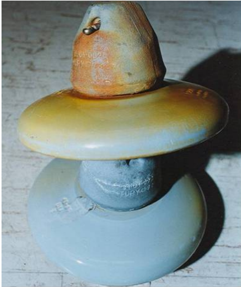
Fig. 3: Flashed porcelain cap and pin suspension insulators from a mining location in the USA. Contamination was suspected as the root-cause, but except for hardware staining on the top bell, the rest of the bells look fairly clean (ESDD measured <0.05 \text{ mg/cm}^2 ).
