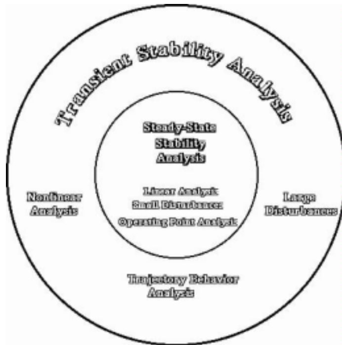
Figure 1. Transient and Steady-State Stability
