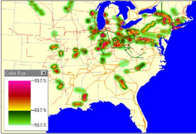
Figure 7: Eastern Interconnection Line Loading Contour
