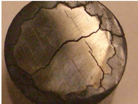
Figure 2.5: The cross-section of the sample kept in furnace for 15 days at 200 °C
