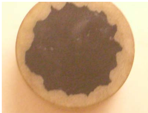
Figure 2.3: The cross-section of a new carbon composite core sample
