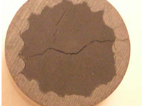
Figure 2.4: The cross-section of the sample kept in furnace for 5 days at 175 °C
