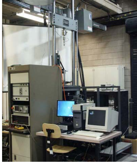
Figure 5.1: Tensile testing system
