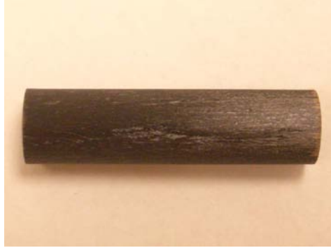
Figure 2.6: An aged sample showing the polymer resin of the carbon composite core
