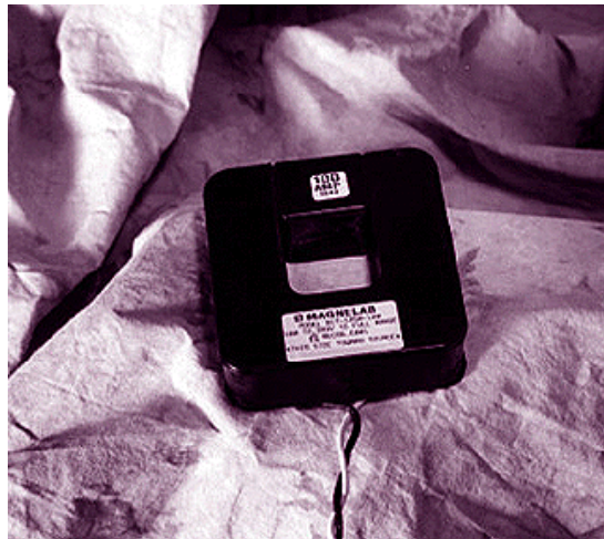
Figure 4.4: Current transformer used to monitor currents in coils, pumps, and fans
